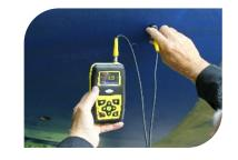
All probes have Intelligent Probe Recognition (IPR), which automatically adjusts settings in the gauge at the same time as transmitting recognition data - the result is a perfectly matched probe and gauge for enhanced performance.
